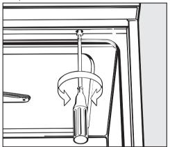
Screw the washer to the countertop through the left and right holes in the front trim.
